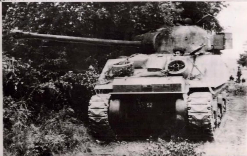
ABOVE: A news wirephoto Sherman Firefly with its powerful 76.2mm 17-pounder anti-tank gun behind one of Normandy's many hedges. The Firefly was soon highly valued, as its gun could penetrate the armour of the Pzkwf V Panther and Pzkwf VI Tiger tanks the allies faced in Normandy
